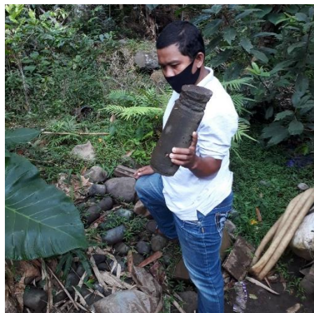
Figure 5. Drilled Breccia Rock
